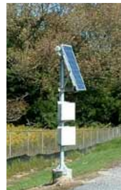
▲ Solar-powered site boundary radiation monitor.
